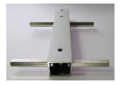
The next step is to mount the OMS-boards to both sides. Therefore you have to place the square-profile as shown in the image (page 16). The top side of the square-profile can be easily identified: the large boreholes for the motors are closer to the top side of the profile.
