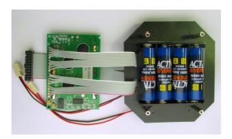
If required the batteries of the bottom side can be fixed by the enclosed cable ties. Therefore the two cable ties have to be spanned through the four remaining boreholes around both battery packs.
