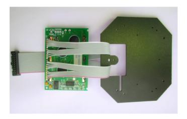
Before the upper battery pack is screwed at the boreholes (2) with the 5 mm recessed head screws (M2x5) the connector must be put through the cable cut-out.
