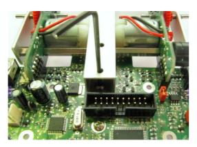
with a pincer from inside through the both front bore holes of the square-profile. Now the engine section is fixed with the two 10-way headers of the OMS-boards to the main circuit board. Pay attention that the both hexagon socket screws inserted before, are put through the board after the assembly. These two screws are now fixed from the bottom side of the board each with a plastic grommet (for not to damage the board) and a nut. Using the
