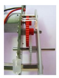
Finally a 25 mm bolt is fixed with a hexagon socket screw to the top side of the square-profile:
