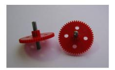
Now the both white double gearwheels have to be pressed onto the two long steel axes (3x37 mm). The distance from the smaller gear to the end of the axis should be 17 mm:
