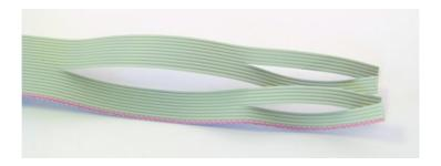
Now each conductor needs to be separated (approx. 2 cm), isolated (approx. 5 mm) and tinned. Afterwards you may solder five conductors in each step.
