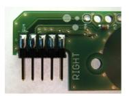
The 10-way headers are soldered with their shorter pins onto the OMS-boards (see the photo left side).
