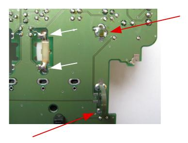
Then the motor contacts have to be soldered to the board (white arrows).
