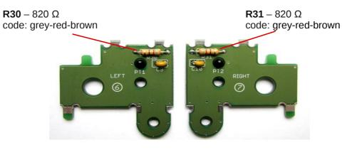
*Hint:* The resistors and the capacitors on the boards **(a)** and **(c)** have to be soldered plain onto the boards, so that they don't interfere with the driving unit in the end!
