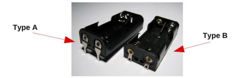
**Before assembling** the packs you have to pay attention to the "+/-" labels on the circuit board and to the "+/-" labels of the respective battery pack (the important side is the **side with the soldering contacts**: the outside contact plates).
