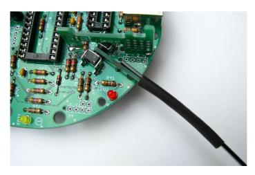
While shrinking the soldering iron should have at least 3 mm distance to the heat-shrinkable tubing.
