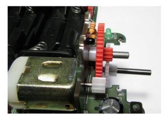
The transmission is fixed by the board @ (the electronic parts of the board @ point inwards). Finally the covering plate is pressed onto the boards @ and @ with careful pressure (see image).
