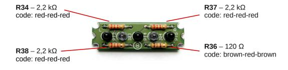
The following overview diagram simplifies the placement of the resistors to the main circuit board. All resistors are shaded light grey, are thickly bordered and contain their specific value.
