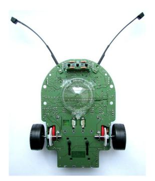
Finally the big half sphere must be put onto the NIBObee – now the robot is ready for takeoff!
