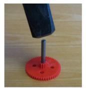
Then you have to press the axis **carefully** with the small hammer through the gear. Afterwards the gearwheel should be in the middle of the axis:
