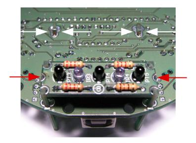
Now the mechanical assembly should be fixed. Finally the remaining contacts have to be soldered on **both sides** (all in all **12** contacts):
