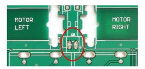
**2.** Jumper for a firmware update of the ATtiny44: With the jumper JP4 it is possible to make a firmware update of the ATtiny44 by the ATmega16.
