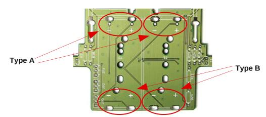
The "+/-" labels of the board and of the pack **only** has to suit at the **side with the soldering contacts**.
