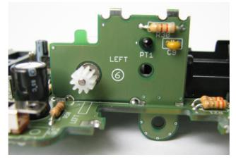
The soldering contacts of the motor have to fit exactly into the recess of the main circuit board:
