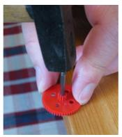
Now the both **white** double gearwheels have to be pressed onto the two **long** steel axes (3x37 mm). Therefore you have to press the axis with the help of a small hammer into the side of the gearwheel with the **smaller** gear.
