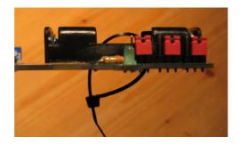
Then the cable strap is to be fastened:
