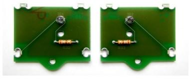
The circuit boards (2) and (3) have to be soldered from the **bottom side**:
