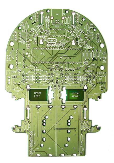
All boards must be separated from the frame first e.g. by a universal pliers:
