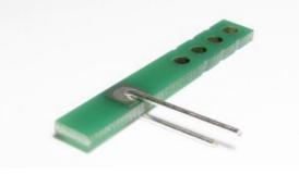
The wire must be soldered to the contacts of the board on both sides. Then it has to be put through the boreholes of the main circuit board:
