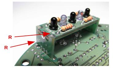
If everything is **well aligned**, the boards are now fixed by soldering. First of all just the both **middle placed** soldering points of the board **(red arrows)**. Then the boards **(a)** and **(b)** are soldered with the main circuit board (white arrows).
