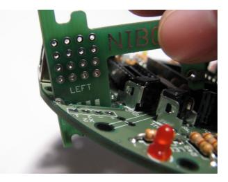
Now the board (a) must be pressed on from the bottom side. Therefore you hold the boards (a) and (b), turn the main circuit board and press the board (b) on so that you can see the electronic parts of the board (b).
