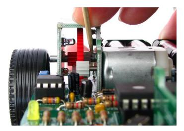
Additional the axis of the white wheels can be greased:
