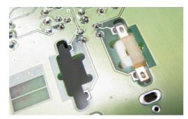
As soon as the motor fits correctly the board (6) is soldered to the main circuit board beginning with the middle soldering contact (see pictures).
