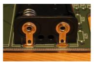
The soldering contacts of the battery packs of **type A** must point to the **middle** of the main **circuit board**.
